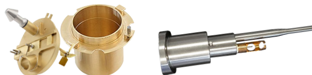
Figure 2: ABA 4 standard test cup with lid and multi-detector
