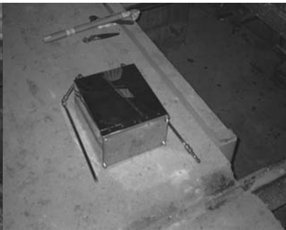
Inlet and overflow points piped to the front of the kiln car.
