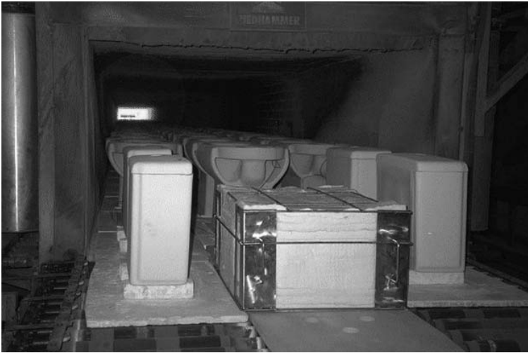
Tracker system entering the kiln.
