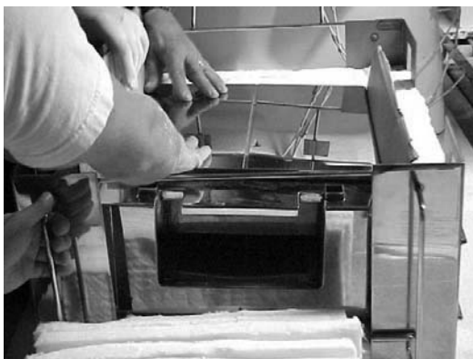
Placing the thermal barrier within the insulation layers.
