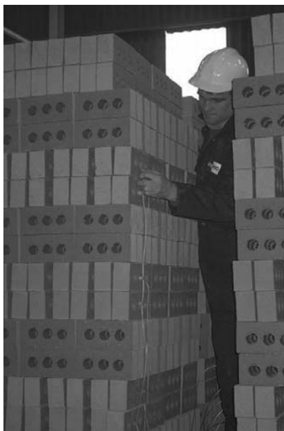
A Kiln Tracker System ready to monitor bricks during firing.
