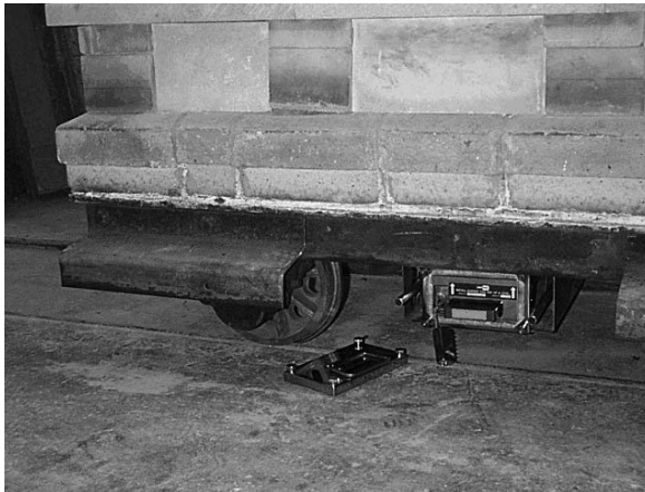
Thermal Barrier in place on the underside of a kiln car with part of the 'skirt' removed for fitting.
