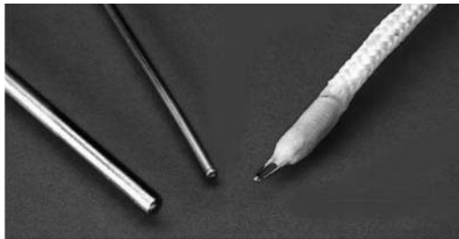
Detailed view of thermocouple hot junctions.
