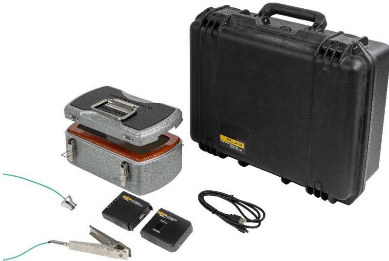
Figure 1-1: A typical Oven Tracker Datapaq XL2 system
