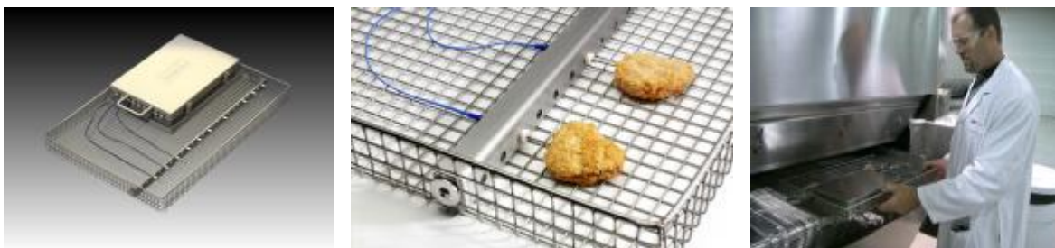
Fig 8: Datapaq Food Tracker profile tray used for repeatable monitoring of conveyORIZED cook processes quickly and efficiently.
