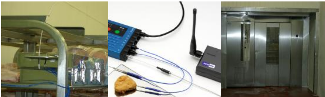
Fig 7: (a) Food Tracker RF system installed on food rack showing external transmitter aerial which sends data straight back to the monitoring PC. (b) Data logger with RF aerial and receiver unit (c) Rotational batch roasting oven into which the product rack is wheeled. Transmission of temperature data, both product and air, from inside the oven is possible without any need for trailing thermocouples which would be impossible if any rack rotation is employed.
