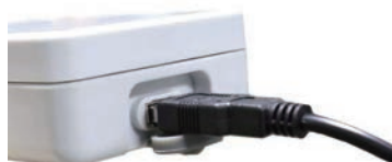
USB Data Output & Power Supply
